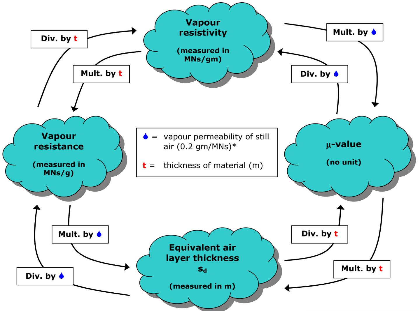
\*This value of 0.2gm/MNs is used by convention in the UK. Outside the UK, local values for atmospheric temperature and pressure can be used to calculate the vapour permeability of still air from basic principles.
